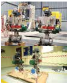
TRUNNION MOUNTED BALL VALVES Class – 150# through 2500# Size 2" through 48"
